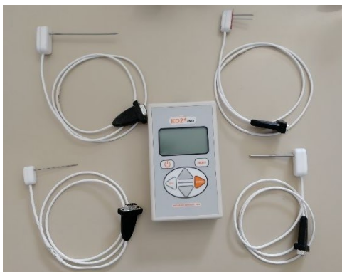
Figure 10: Example of a needle probe device (KD-2) used for sediment measurements.
