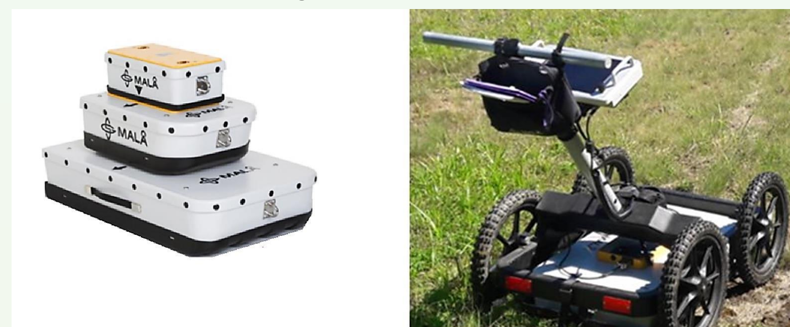
Figure 1: GPR equipment used. Left – 250, 500 and 800 MHz antennas; Right – GPR cart with 250 MHz antenna, operating unit and monitor.
