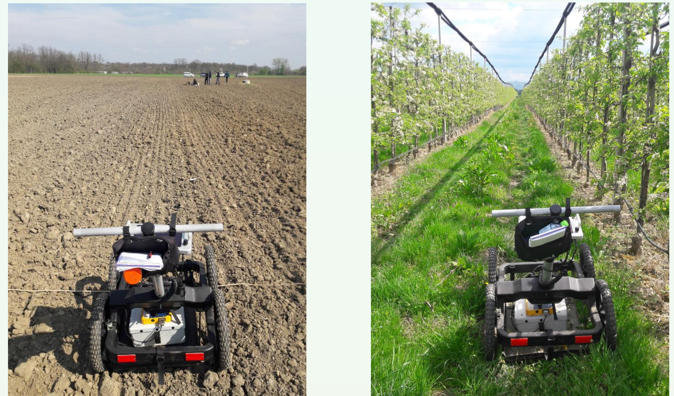
Figure 1: Measurement with a GPR cart and 500 MHz antenna on an empty field (left) and in an orchard (right).
