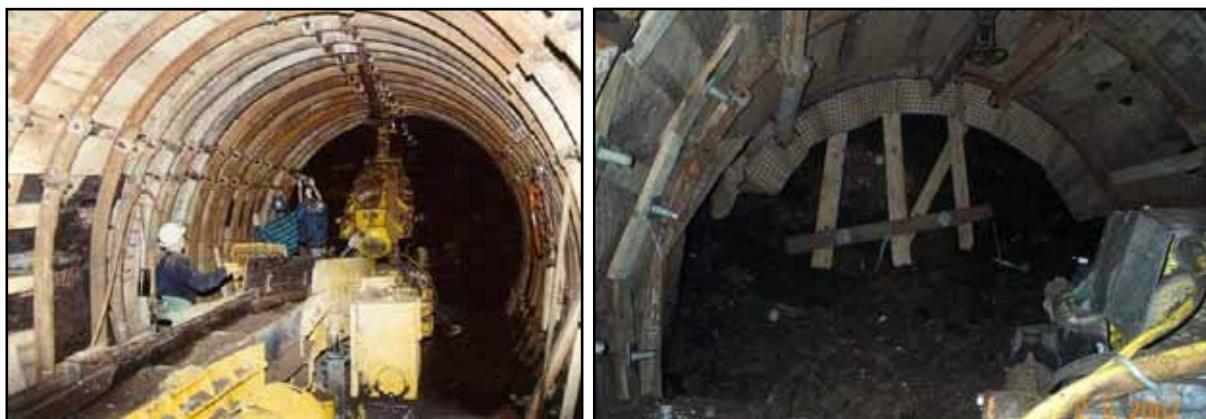
Fig. 6.27: Two mining road-faces, ca 4×4 m wide. The sidewalls are covered by wooden planks.
