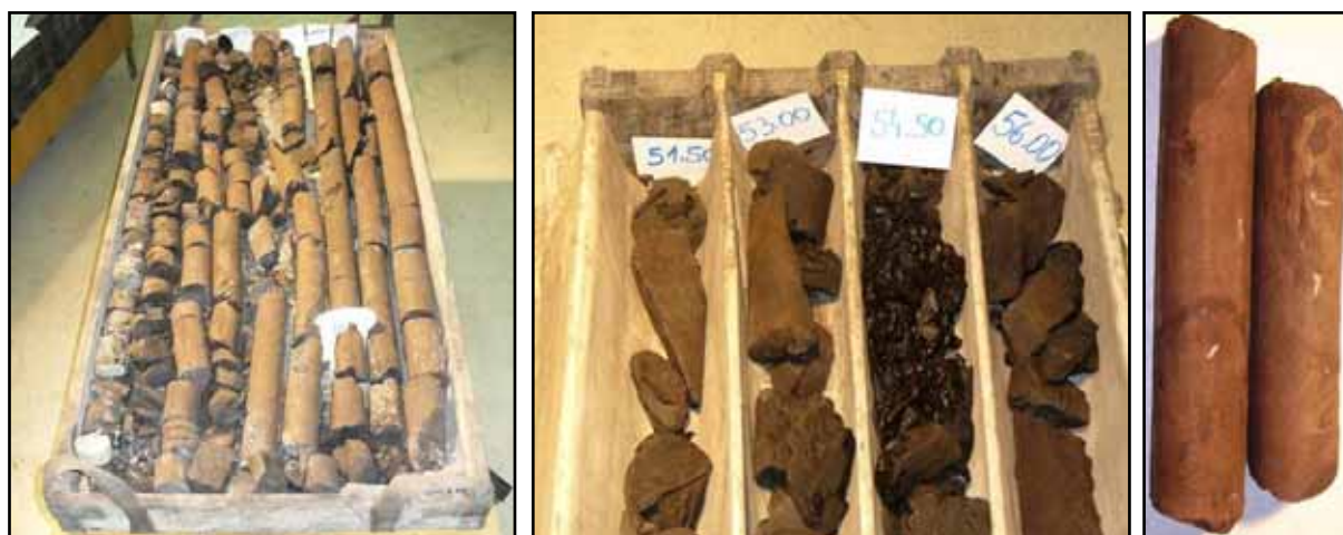
Fig. 6.1: Lignite core from an underground borehole (JH-3/06). Note differences in “rock quality” (crushed versus compact core). Box length is 1.5 m, core diameter is 54 mm. The right photo shows a ca. 35 cm long xylite-rich core segment with white calcite “inclusions” (borehole JH-3/06 at 62.00 m length).
